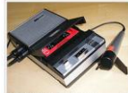
One of the first (portable) cassette recorders from Philips, the Typ EL 3002 (1968)
