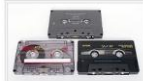
Cassettes of varying tape quality and playing time. The top is a Maxell MX (Type II), bottom right is a TDK SA (Type II) and the bottom left is a TDK D (Type I).
